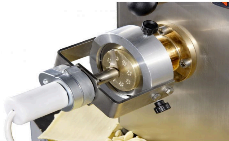
Optional variable speed rotary cutter for short pasta
