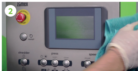
2 The sections of the control panel should be washed with a damp cloth, since it is susceptible to splashing.*
