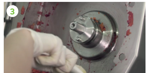
3 We open the feeding hopper and with water we drive all the pulp towards the exit mouth.
